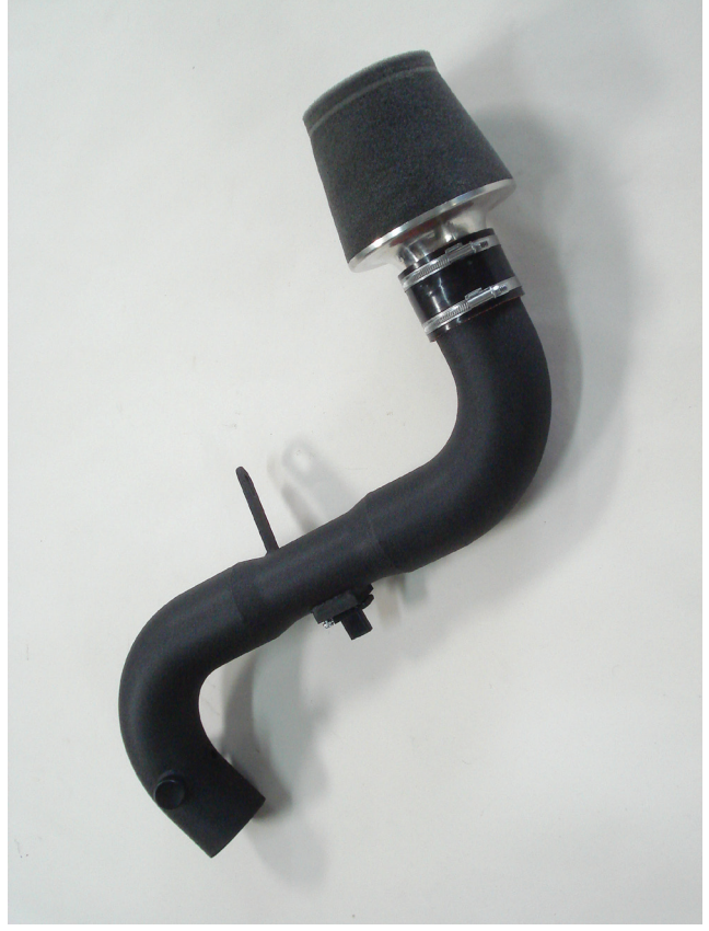
Figure 8. FSWerks Intake ready for installation.
