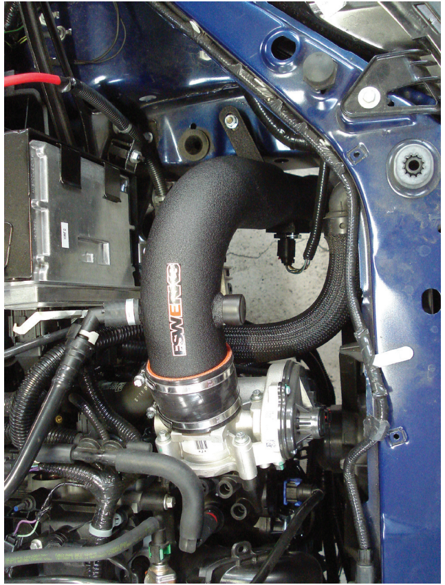
Figure 11. Intake installed properly.
